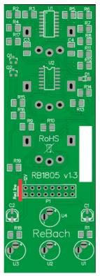
Connect the power cable with the red band facing to the left side of the module (rear view)
